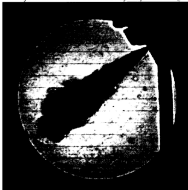
Figure 1 Typical shadowgraph of a diesel fuel injection
